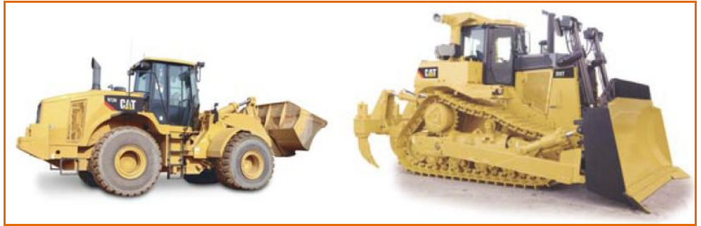
Exhibit 3 : 972H Wheel Loader (left) and D10 Dozer (right) for Mining at Barnes Hill
